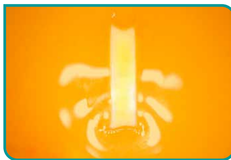
Fig. 2: An example of good shape of coagulation, good edge sharpness and good homogeneity
