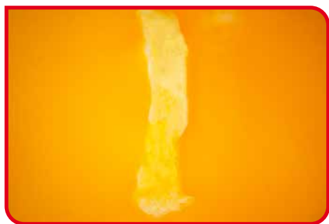
Fig. 1: An example of poor shape of coagulation, poor edge sharpness and poor homogeneity
